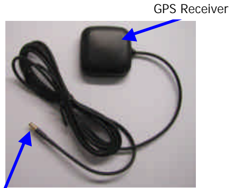
MCX Connector, plugs into the back of Road Angel
